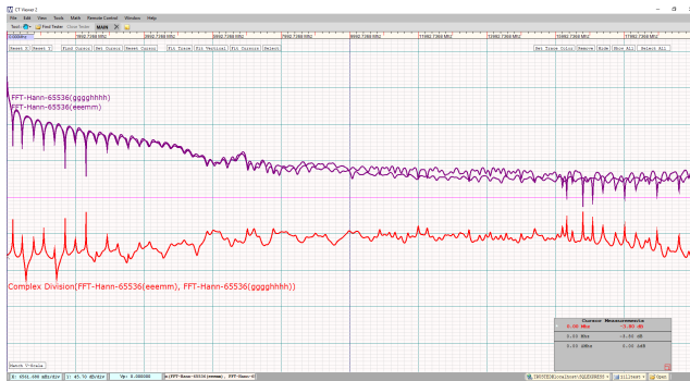
Figure 5.37 Getting the Complex Division of two FFT traces. The Complex Division is shown in red.
