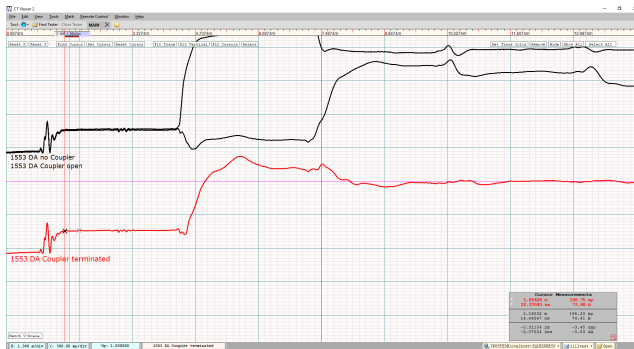
Figure 5.4 Use Shift-S to move only the selected trace down relative to the other traces.
