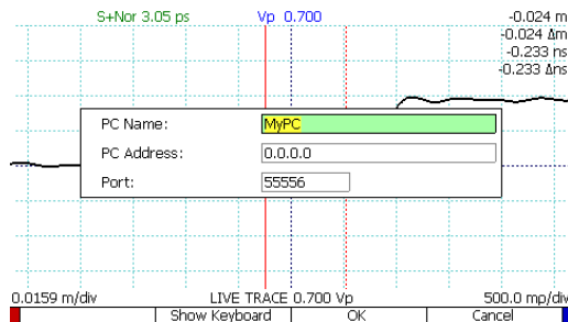
Figure 3.11 After selecting Add PC , enter the information for the PC into this dialog box.
