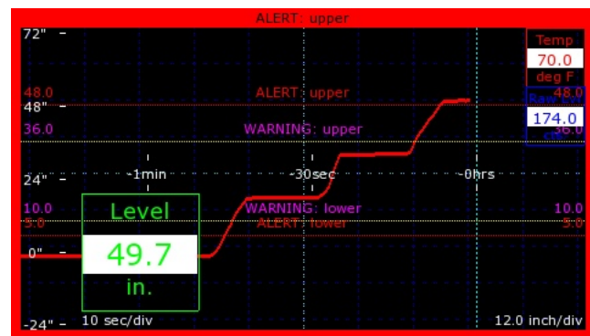
EFP-HL real-time level history graph with level alarms.
